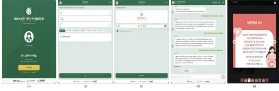
Figure 6. The deployed DU-AI counseling interface, showing (a) the landing screen, (b) on-device client-profile onboarding, (c) the knowledge-base (RAG) panel with 4,839 indexed chunks, (d) a counseling session with retrieval-attached educational media, and (e) the full-screen media viewer.
