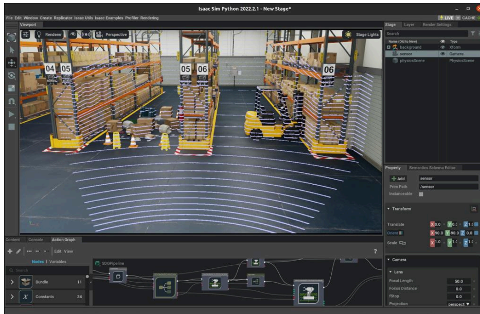
Figure 1. Indoor AMR Simulation Environment Using NVIDIA Isaac Sim
